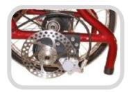
Anti Roll Back, Wheelchair will not roll backwards down an incline while Transmission is engaged. Front Wheel suspension giving lateral stability, reduced shock loading.
